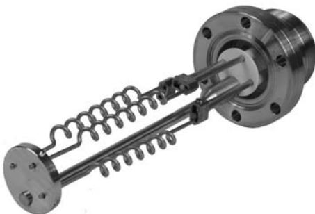
The filament cartridge is mounted on a 2- 3/4" CFF (NW 35). The feedthrough supports three titanium-molybdenum filaments and a return path for ground isolation. Each filament contains 1.5 grams of usable titanium and averages 20 hours of operation.
