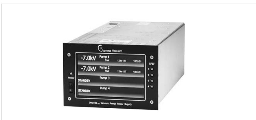
Ion pumps 100 l/s and larger required higher currents for starting and higher pressure operation. The QPCe supplies up to four ion pumps with 125 mA (125 watts) each. The easy-to-read color touchscreen display simultaneously displays pressure, current, and voltage. Standard serial and standard Ethernet communications along with legacy set-point and analog outputs allow for easy system integration. The QPCe fits into any rack at just 3U high and 1/2 rack wide.
