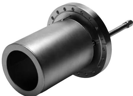
The liquid cryoshroud consists of a double walled, type 304L stainless steel cylinder with two liquid nitrogen feedthroughs with flare type fittings. It provides 1578 cm<sup>2</sup> (245 in.<sup>2</sup>) of liquid nitrogen cooled surface area that provides pumping speeds up to 12,000 l/s for hydrogen (see table). The shroud is mounted on an 8 in. CFF (DN 160) or 10 in. CFF (DN 200)
