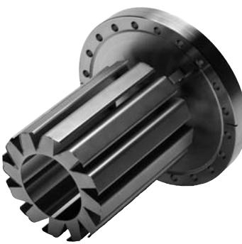
The ambient sputter shield economically maximizes surface area when cooling is not practical or possible. It provides 827cm<sup>2</sup> (128 in.<sup>2</sup>) of ambient temperature surface area that provides pumping speeds up to 2,200 l/s for hydrogen (see table). The shield is mounted on an 8 in. CFF (DN 160) or a 6 in. CFF (DN 100).
