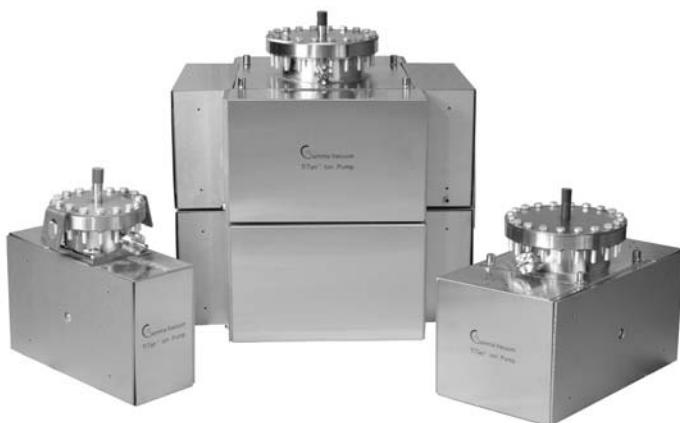
Low Profile ion pumps are under 12 in. (300 mm) high for standard configurations. The closed magnetic loop of these pumps reduces the stray magnetic field created by the pump making these pumps ideal for any type of charged particle application.
