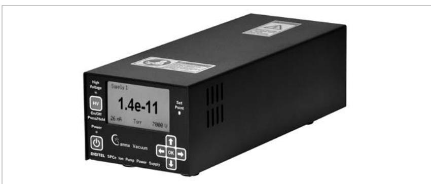
The SPCe is a versatile way to fully operate ion pumps 0.2 – 75 l/s with up to 40 mA (50 watts) of power. An LCD pressure/current/voltage display along with standard serial communications makes the SPCe able to accommodate the needs of basic and advanced users. Nano amp resolution provides gauging capabilities using the appropriate ion pump set-up.
