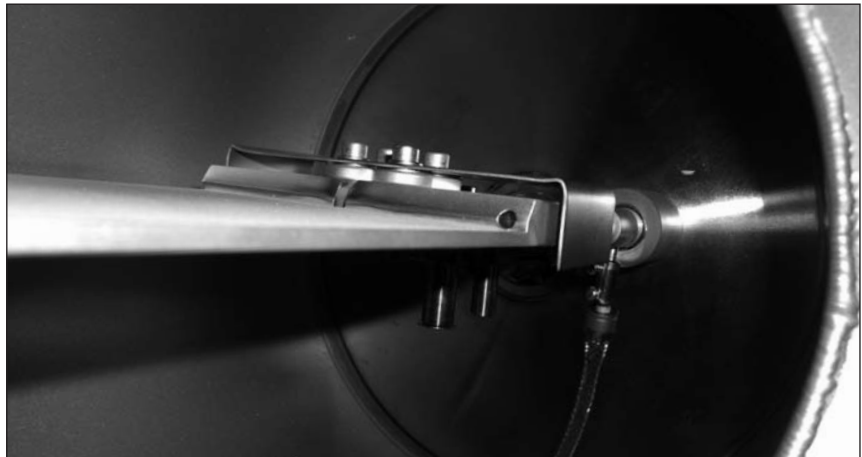
Insulated substrate fork with RF bias connection
