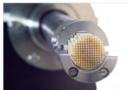
Intra-catalyst sampling of gas and temperature
