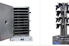
24-Port column manifold for external drying of larger volumes of liquids or slurries in flasks. Includes 24 ports, mounted radially around column with 24 removable neoprene valves, each of which can be fitted with a flask of up to 1 litre capacity (flasks not supplied). A manifold sealing gasket is provided with to seal the base.
