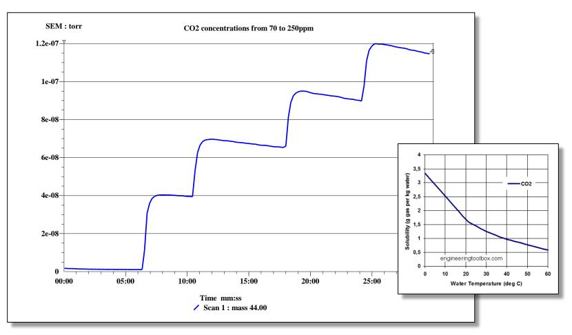
The figure shows the addition of 10mL aliquots of a  $CO_2$ -satured  $H_2O$  solution (1.5g  $CO_2$  per 1 kg  $H_2O$  at 23 °C as per inset graph) to 200 mL pure  $H_2O$ . Therefore, the concentrations of  $CO_2$  are approximately 0, 70 ,140, 200, and 250 ppm for the 5 time steps shown.
