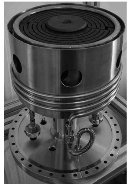
Rotating high temperature thermal radiation heater with SiC heating element
