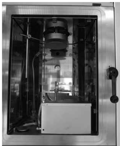
Rotating and water-cooled substrate table
