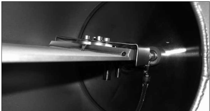
Insulated substrate fork with RF bias connection
