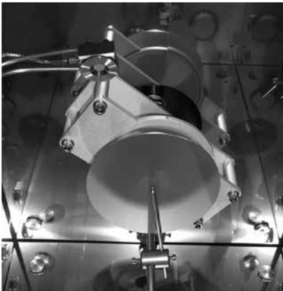
Motor driven rotary drive with a detachable substrate holder (bayonet coupling). View from the bottom onto the closed substrate shutter
