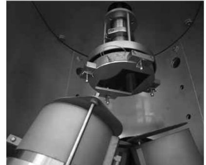
Rotating contact heater based on the resistance heating principle
