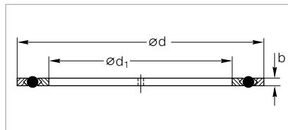
Dimensional drawing for vacuum sealing disks
