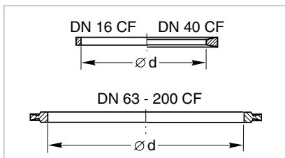
Dimensional drawing for the profiled gaskets
