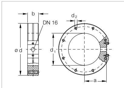
Dimensional drawing for the measurement flanges
