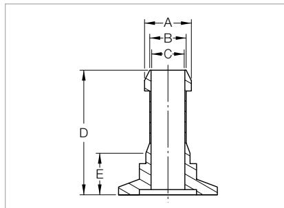
Dimensional drawing for the ISO-KF nipples
