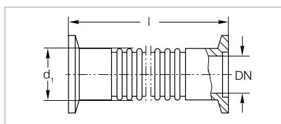
Dimensional drawing for the vacuum hoses with flanges
