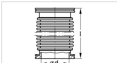
Dimensional drawing for the flexible vacuum hoses
