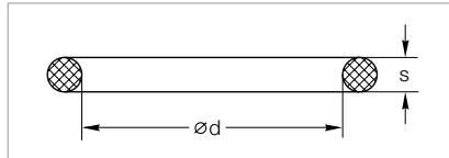
Dimensional drawing for the spare O-ring gaskets for ISO-KF flange connections
