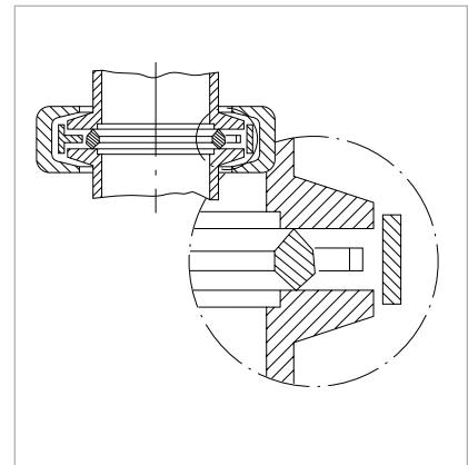
Small flange connection with ultra sealing ring
