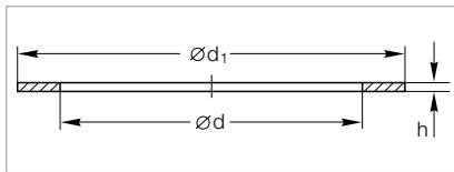
Dimensional drawing for the copper gaskets
