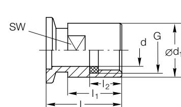
Dimensional drawing for the screw-on flanges
