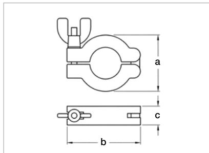
Max. torque at the wing nut: 2 Nm
