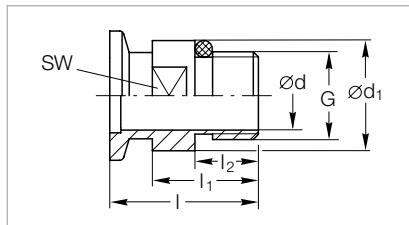
Dimensional drawing for the screw-in flanges
