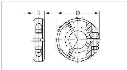
Dimensional drawing for the clamping collars for ultra sealing rings
