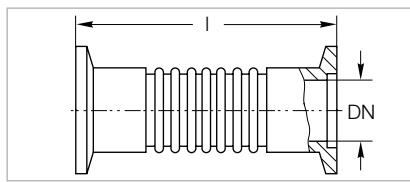
Dimensional drawing for the bellows with flanges
