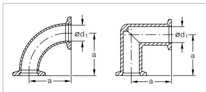
Dimensional drawings for the pipe bends 90° (stainless steel, left) and the mitred elbows 90° (aluminium, right)
