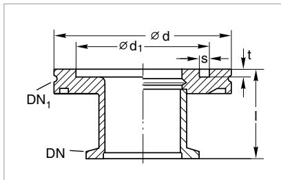
Dimensional drawing for the adaptor reducers ISO-KF – ISO-K;
