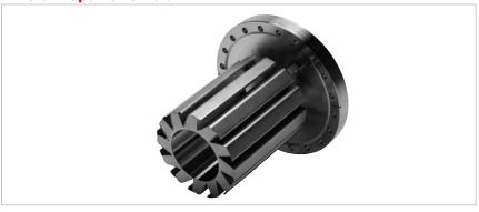
The ambient sputter shield economically maximizes surface area when cooling is not practical or possible. It provides 827cm2 (128 in.²) of ambient temperature surface area that provides pumping speeds up to 2,200 l/s for hydrogen (see table). The shield is mounted on an 8 in. CFF (DN 160) or a 6 in. CFF (DN 100).
