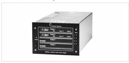
lon pumps 100 l/s and larger required higher currents for starting and higher pressure operation. The QPC supplies up to four ion pumps with 125 mA (125 watts) each. The easy-to-read color touchscreen display simultaneously displays pressure, current, and voltage. Standard serial and standard Ethernet communications along with legacy setpoint and analog outputs allow for easy system integration. The QPC fits into any rack at just 3U high and 1/2 rack wide.
