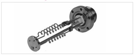
The filament cartridge is mounted on a 2- 3/4" CFF (DN 40 CF). The feed-through supports three titanium-molybdenum filaments and a return path for ground isolation. Each filament contains 1.5 grams of usable titanium and averages 20 hours of operation.
