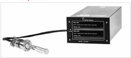
The TSPq controller has an easy-to-read color touchscreen display that displays all manual or programmed firing paramenters. Manual operation is as simple as pressing one button. Programming is just as easy by viewing all programming options on one screen. The TSPq controller can operate up to 8 TSP filaments.
