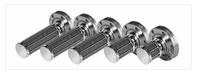
Non-evaporable getter (NEG) pumps operate with a non evaporable, compact getter material with a porous structure. The gas molecules either adsorb on the surface of the getter material or diffuse rapidly into it. The NEG pump contains a heating element which is used for regeneration. The getter material consists of a zirconium-aluminum alloy which allows for
